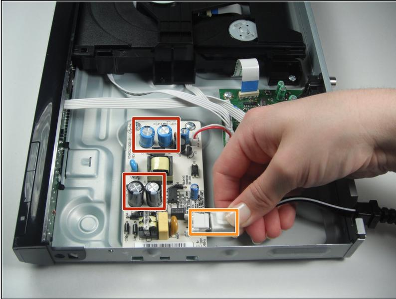
**⚠ Caution:** The circuit board contains capacitors (they look like cylinders) that can shock you if they discharge. Be careful not to touch them as you work. If possible, use a [capacitor discharge probe](#) to safely rid the capacitors of dangerous charges.
