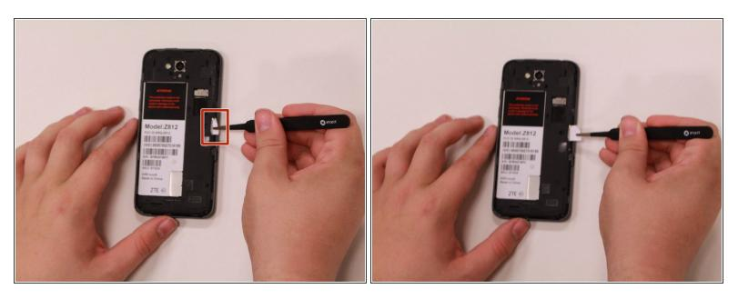
• Remove the SIM card from the right side of the device using a pair of tweezers.
