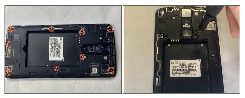
Remove all nine of the 3.0mm screws on the back of the phone using a Phillips #0 screwdriver, including the one attaching the camera lens.
