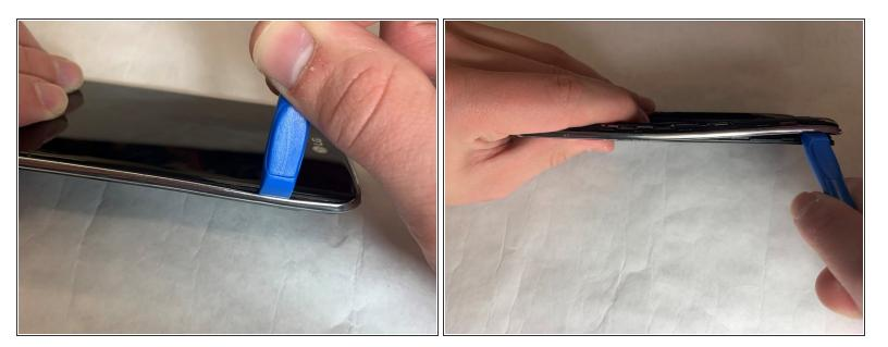
• With the plastic opening tool, pry between the screen and the outer chrome edge to remove the bottom shield from the rest of the phone.
