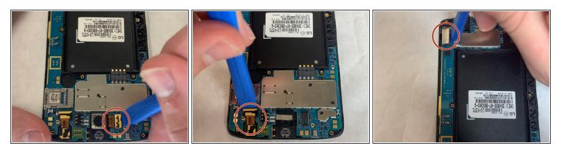
• With a plastic opening tool, disconnect all three ribbon connectors from the motherboard: one for the front camera, one for the rear camera, and one for the screen.
