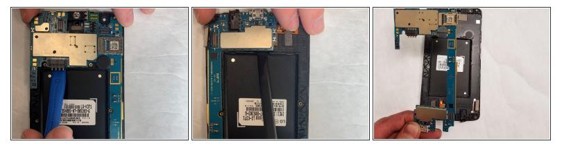
Using a plastic opening tool, separate the motherboard from the back frame and remove it from the device.
