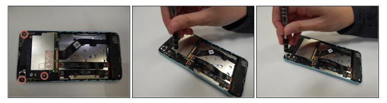
• Use a T5 Torx screwdriver to remove the three 4.0 mm screws.
