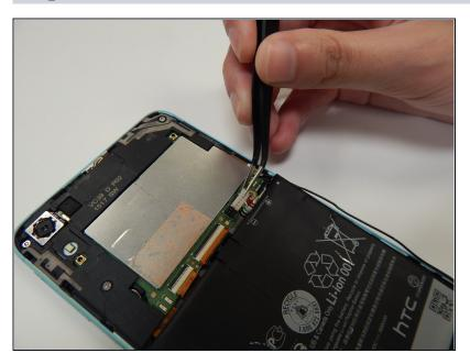
• Disconnect the battery cable from the motherboard with the tweezers.
