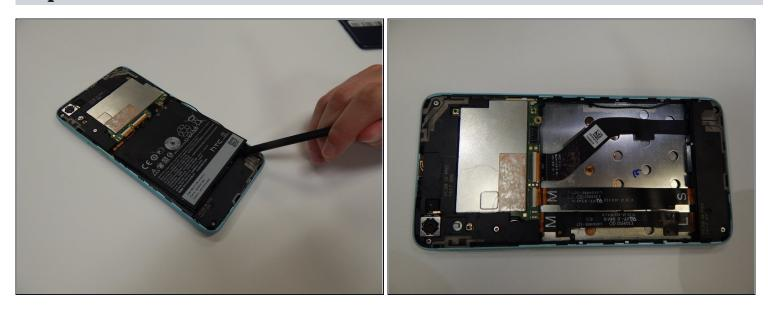
• Lift the battery with a plastic spudger and remove it from the device.
