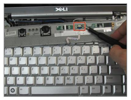
Use <u>tweezers</u> to squeeze the tabs on the connector and remove the ribbon cable.
