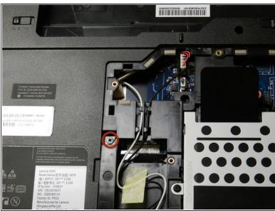
Locate the Optical Drive 4.7 mm Philips #1 screw, which secures the Optical Drive into the body of the laptop.
