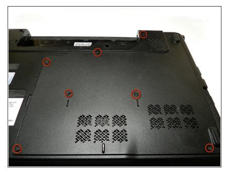
Remove the seven 5.3 mm Phillips #1 screws holding the back panel in place.
