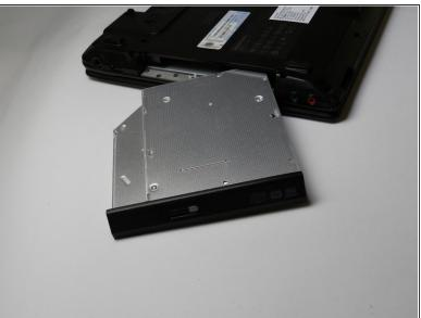
Slide the Optical Drive smoothly out of its slot.
