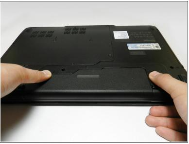
Locate the two switches that lock the battery. Push the right-hand switch outward into the "unlocked" position.
