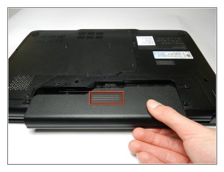
Push and hold the left hand switch outward in the "unlocked" position, then gently slide the battery away from the computer.
