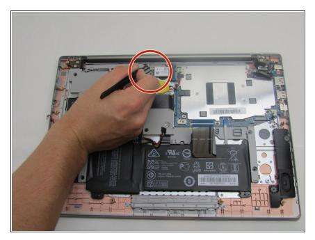
Remove the wireless card by disconnecting the two antenna cables and removing the 2.5 mm Phillips #0 screw.
