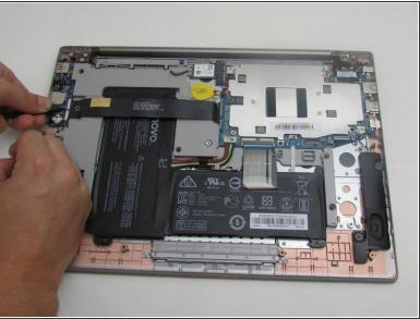
Use a spudger to lift the black fastener and disconnect the ribbon cable from the USB daughterboard.
