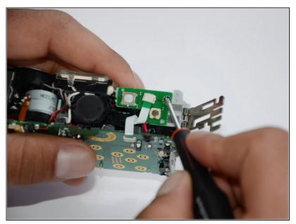
• Remove the 5mm Phillips #00 screw that is located on the top of camera.
