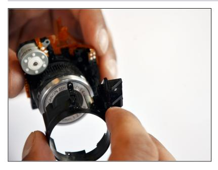
Gently slide off the black piece surrounding the lens. The lens is now disassembled!
