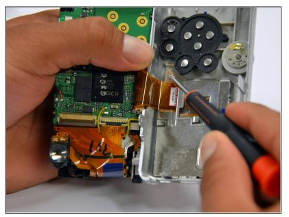
• Remove the 4mm Phillips #00 screw from above the ribbon.
