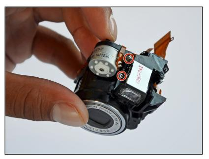
Remove the two 2mm Phillips #00 screws on the top of the lens piece.
