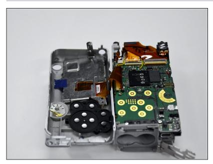
• Gently peel off the blue tape on the top of the LCD screen.
