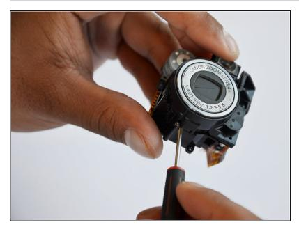
• Remove the 2mm Phillips #00 screw on the bottom of the lens piece.
