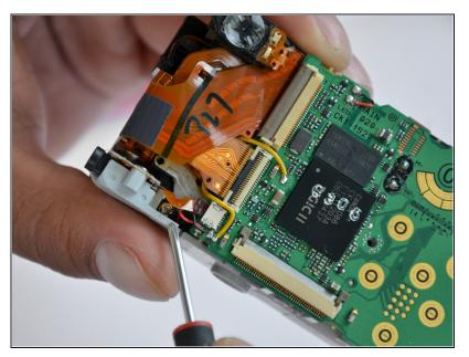
Remove the 5mm Phillips #00 screw near the bottom left of the motherboard.
