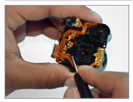
Remove the 5mm Phillips #00 screw on the back of the lens piece.
