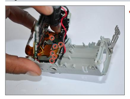
Remove the six 2mm Phillips #00 screws that are located under the motherboard.
