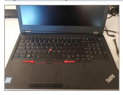
The first step is to remove the track pad left and right click covers. I used a plastic spudger tool to carefully pry and remove.
