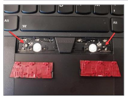
Once you have removed the covers you will see two screws (one on each cover). Using a PH0 screw driver, loosen the screws (they are attached so will not come out).
