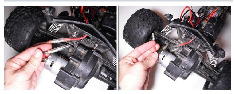
• Pull the black power wire in an outward motion on both sides of the clear plastic sleeve to disconnect the motor from the battery. Repeat this with the red power wire to disconnect it from the battery.
