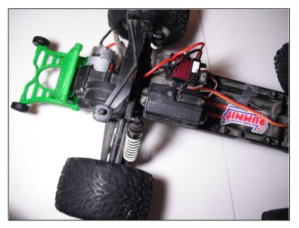
• Lifting straight up, remove the plastic body from the truck, exposing the inner components.
