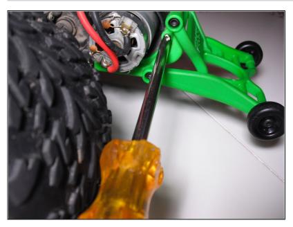
• Using the Phillips #1 screwdriver, remove the center screw on the left side of the green wheelie bar.
