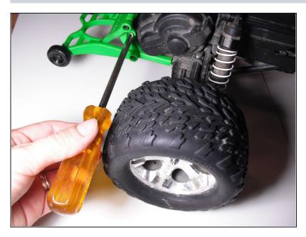
• Using a Phillips #1 screwdriver, on the rear right side, remove the center screw from the green wheelie bar.
