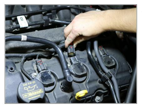
Pull the red tab out of the electrical connector and slide the connector off of the coil pack.
