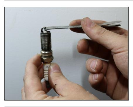
Check the spark plug gap using the spark plug gap gauge. Make sure the gap is within desired specifications.
