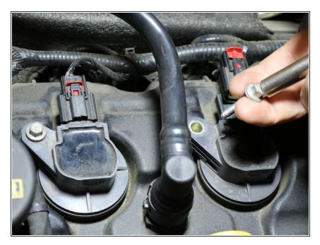
Remove the 10mm screw from the coil pack. Use the 10mm socket on the 3/8" drive ratchet to remove the screw.
