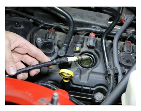
Remove the spark plug from the cylinder using the grabber tool.
