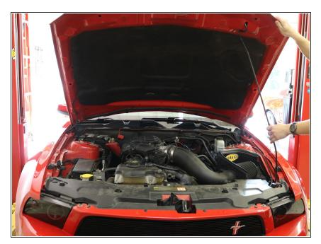
Open the hood and prop it open using the hood prop.
