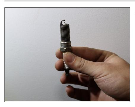
Inspect the spark plug for blackening or other damage.
