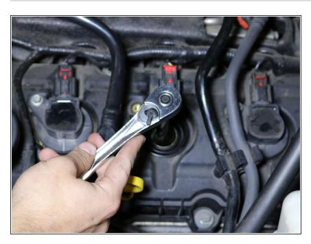
Loosen the spark plug completely using the 3/8" ratchet and extension with the 5/8" spark plug socket.
