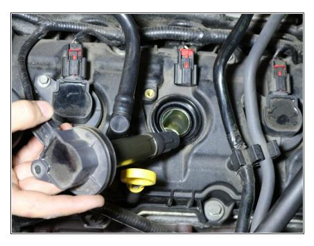
Remove the coil pack from cylinder.
