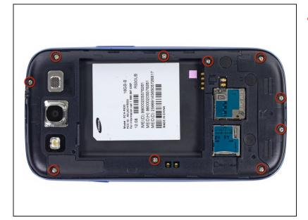
Remove the ten 4.0 mm Phillips screws securing the midframe to the front panel assembly.
