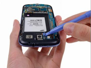
• Use a plastic opening tool to pry the rear-facing camera connector up from its socket on the motherboard.
