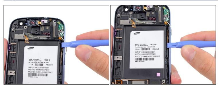
• Wedge the flat edge of a plastic opening tool in between the the earpiece/buttons/ambient light sensor ribbon cable and run it down to loosen the adhesive securing the ribbon cable.
