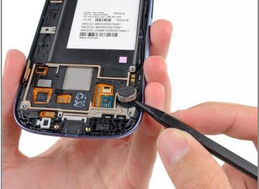
• Use the tip of a spudger to pry the vibrator out of its recess in the front panel assembly.
