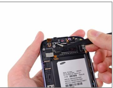
• Use a pair of <u>tweezers</u> to lift the front-facing camera/ambient light sensor/rear microphone assembly out from its socket in the front panel assembly.
