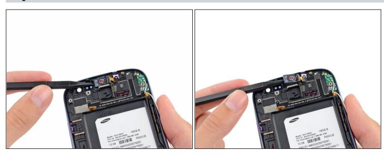
• Wedge the tip of a spudger underneath the earpiece speaker and pry the earpiece speaker out of its recess in the front panel assembly.
