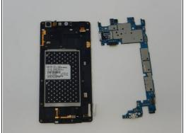
Using the iFixit opening tool, remove the motherboard from the screen by inserting the opening tool under the edge of the motherboard and lifting up.
