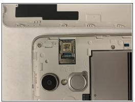
Remove the SD and SIM cards by sliding the cards out with your finger.
