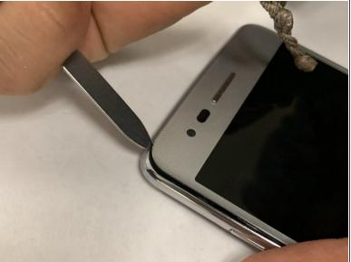
Pry up on the screen with a plastic opening tool.
