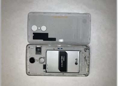
Use an iFixit opening tool to pry off the back case.
