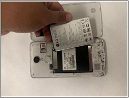
Remove the battery by prying it up with a fingernail or opening tool from the bottom edge.
