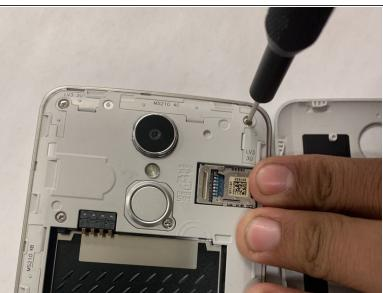
Remove the ten screws from the midframe with a Phillips #000 screwdriver.
