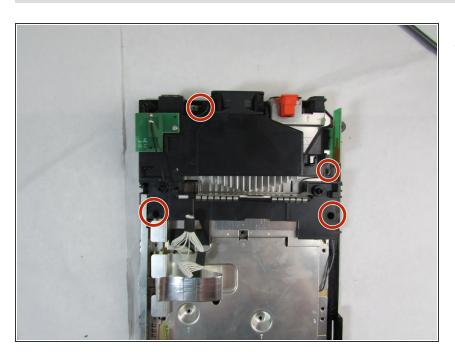
Remove the four black 10 mm screws attached to the black plastic frames using the Phillips #0 screwdriver.
