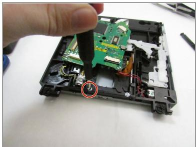
Remove the screw using a Phillips screwdriver.
