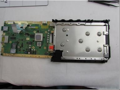
• Once the heatsink is removed, cautiously pull the motherboard out from the left side of the console case and remove it from the device.
