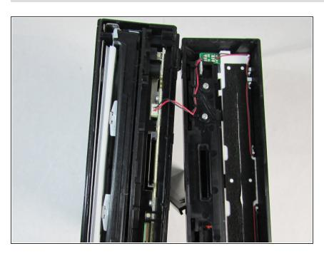
Carefully pull off the front cover (the one with the disc drive hole). You will expose a red and black wire.
