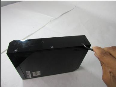
Use tweezers to remove the three black square stickers on the top of the console by prying under and gently pulling up to expose three screws.
