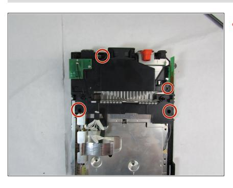
Remove the four black 10 mm screws attached to the black plastic frames using the Phillips #0 screwdriver.
