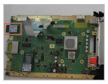
Using your fingers, gently lift and remove the bluetooth module from the motherboard.
