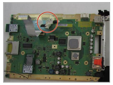
Pull the power supply cable parallel to the motherboard and disconnect it from the device.
