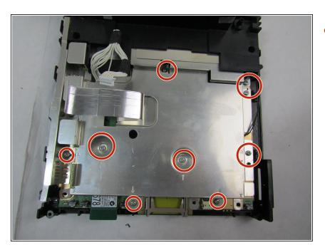
Remove the eight 7mm screws using the Phillips #0 screwdriver.
