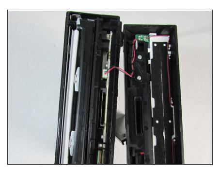
Carefully pull off the front cover (the one with the disc drive hole). You will expose a red and black wire.
