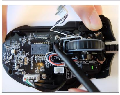
Pry and remove the scroll wheel feedback bar from its hold-down clips using the hook end of a halberd spudger.
