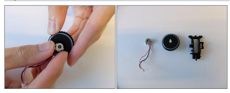
• Remove the scroll wheel optical encoder from the scroll wheel.
