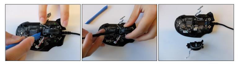
Using the opening tool, pry the black bracket holding the scroll wheel in place backwards until the scroll wheel housing pops out.
