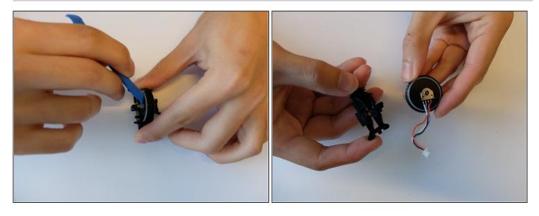
• Remove the scroll wheel from the scroll wheel housing using the opening tool.
