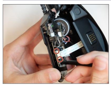
Unlock the ribbon connector that is held down by the main board clips using the spudger's pointed end.
