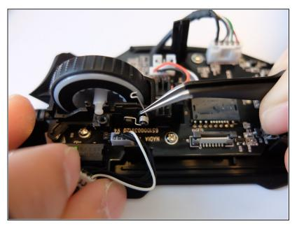
Remove the scroll wheel feedback bar from the scroll wheel by holding down the spring and using angled tweezers to remove it from its placement.
