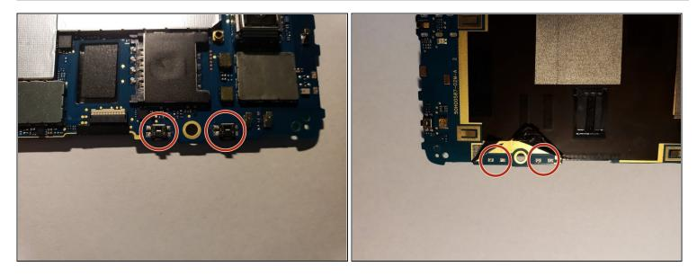
• Desolder the volume buttons off of the motherboard.
