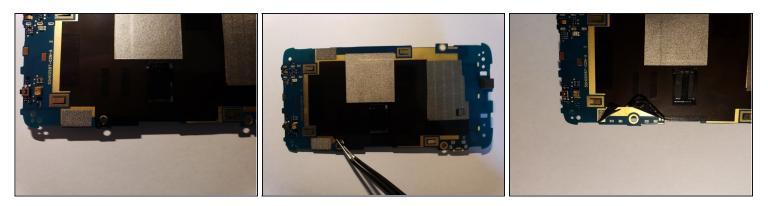
• Peel back the protective tape with <u>tweezers</u> to expose the solder.
