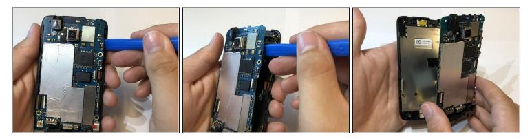
• Use the iFixit opening tool to separate the motherboard from the display assembly.
