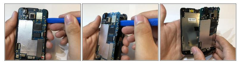
• Use the iFixit opening tool to separate the motherboard from the display assembly.
