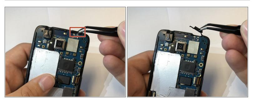
• Remove power button from the top of the phone with tweezers.
