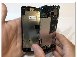
• Use the iFixit opening tool to separate the motherboard from the display assembly.
