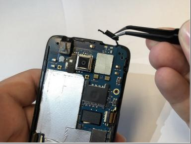
Remove power button from the top of the phone with tweezers.
