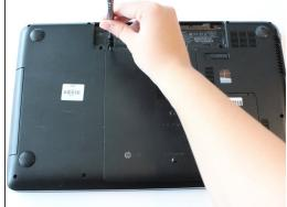
Remove the 6.25 mm screw in the left-lower hand corner of the battery port using a Phillips head screw driver.
