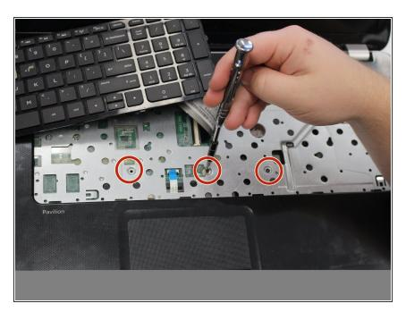
Remove three 6.5 mm Phillips screws located underneath the keyboard using a Phillips #0 screwdriver.
