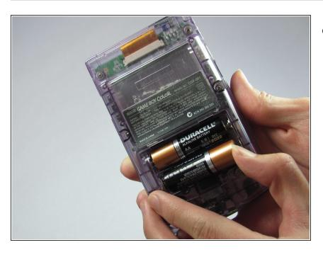
Remove the batteries from the battery compartment.
