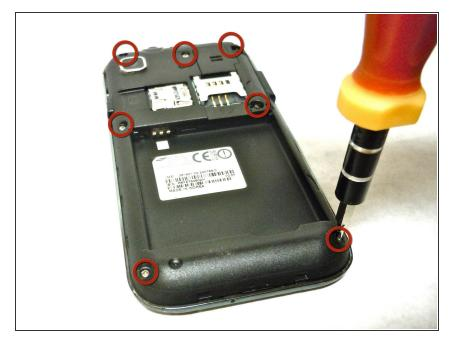
Remove the seven 4.5 mm Phillips #00 screws along the perimeter of the phone.
