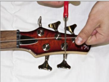
• On a taut string, measure one inch past the nut before using a pair of wire cutters to cut the string.
