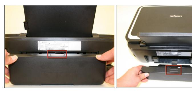
Remove the duplex unit from the back of the printer with the duplex unit facing up.
