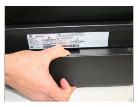
Hold the button down with the flat end away from the printer. When you hear a click, the duplex unit can be removed from the printer.
