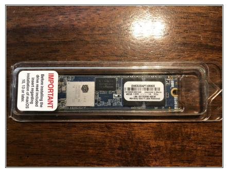
Don't remove from package until we are ready to install it. The lease amount of handling possible ensures no static discharge or other damage can occur.
