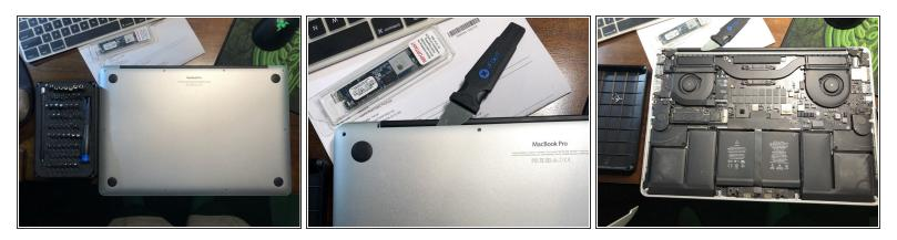
• Shut computer down and flip over to remove back. Use the P5 star tip to remove screws. Place them in a safe, none slip container. These screws are really tiny. Also, the screws closest to the monitor are the shortest and must be separated to ensure they go back in same slot. Otherwise you will have screws stick out in these slots.
