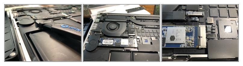
• A Torx T4 bit is needed to remove the screw holding the current SSD card in. Only pry the SSD up this much to remove it. It will be harder to put the new one in vs taking the old one out. Don't worry, it is the right part. Also, be sure to fully seat the new SSD. Failure to do so will cause the drive not to show up in the next step. See pic.
