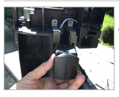
The inner part of the coffee spout is attached with a bayonet. Use a fair amount of force to push the coffee dispenser up and then pull it out away from the machine.
