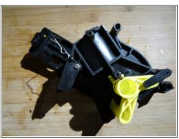
• There are three Torx T10 screws in deep blind holes that hold together the two parts of the brewing unit. Unscrew them and lift off the upper side panel.
