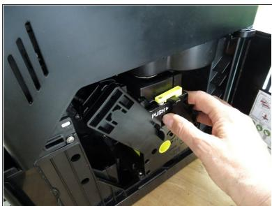
Open the hatch on the side panel and remove the brewing unit.
