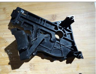
Now you can disassemble the brewing unit into its three main parts: the brewing unit and the two side panels.
