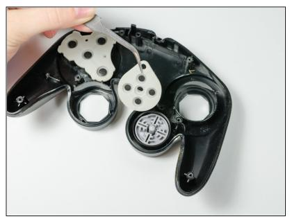
• Remove the rubber backing with <u>tweezers</u>.
