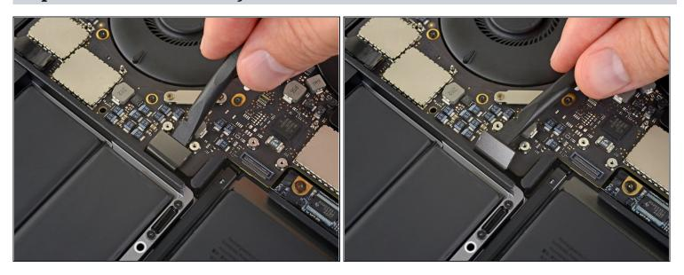
Use a spudger to disconnect the keyboard connector by prying it straight up from the logic board.
