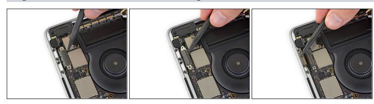
• Use a spudger to disconnect the left-side Thunderbolt port connector by prying it straight up from the logic board.
