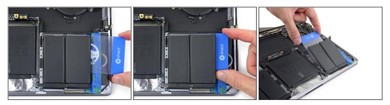
• Repeat the previous two steps to separate the remaining battery cell on the right.
