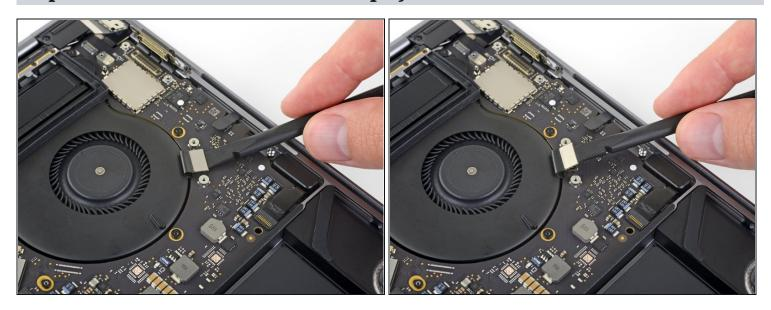
• Use a spudger to disconnect the Touch Bar display connector by prying it straight up from the logic board.
