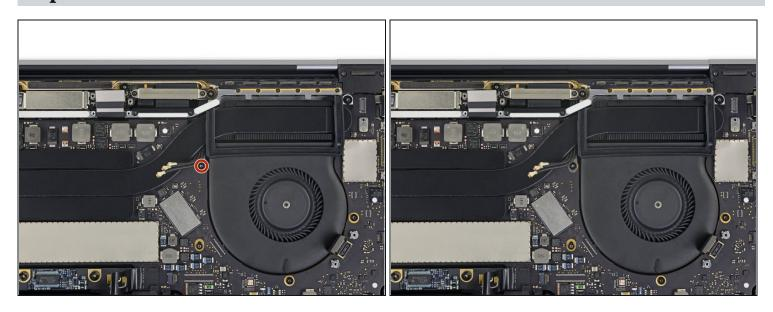
• Use a T5 Torx driver to remove the 2.9 mm screw securing the antenna cable bundle.
