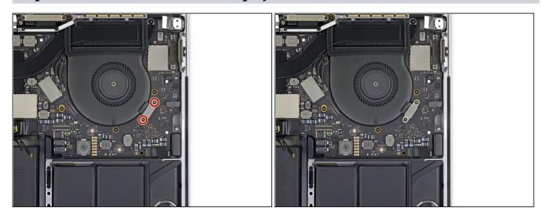
• Use a T3 Torx driver to remove two 1.9 mm screws from the Touch Bar display connector bracket.
