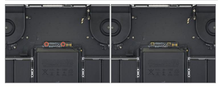
Use a T5 Torx driver to remove the two 3.2 mm screws from the battery board.
