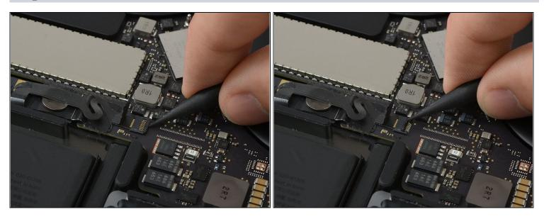
• Use the tip of a spudger to flip up the small black locking tab securing the cable in its connector.
