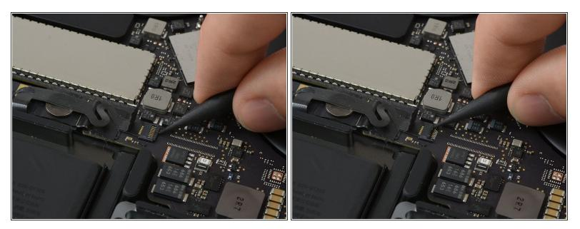
• Use the tip of a spudger to flip up the small black locking tab securing the cable in its connector.
