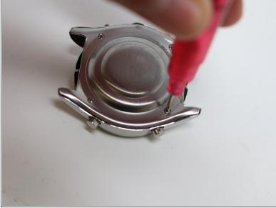
• Remove the four 1.1 mm screws holding the back panel in place using the Phillips #00 screwdriver.
