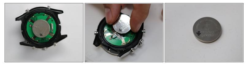
• Remove the large circular Analog battery.
