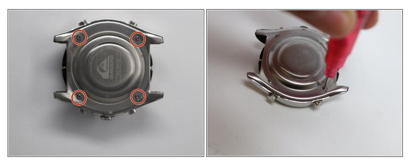
• Remove the four 1.1 mm screws holding the back panel in place using the Phillips #00 screwdriver.
