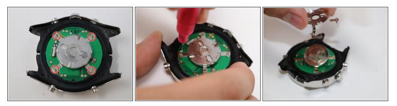
• Remove the four 1.1 mm screws located on the metallic holder using the Phillips #00 screwdriver.
