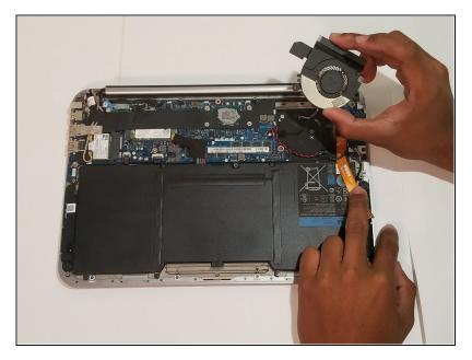
• The cooling fan can now be removed and a new one can be installed.
