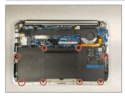
• Use a Phillips #00 screwdriver to remove the 8 screws that secure the battery.
