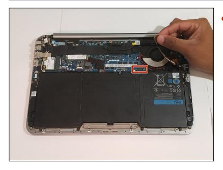
Disconnect yellow-colored ribbon cable from its port which sits at the bottom left of the fan housing.
