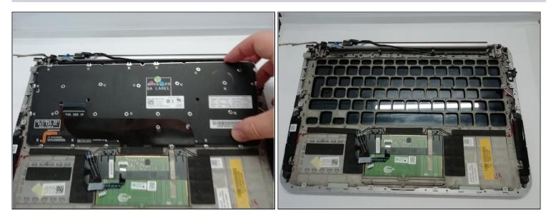
• You can now remove the keyboard. And also do a cleaning if necessary, as in the second photo.
