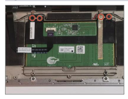
• Use a Phillips screwdriver to remove the 4 trackpad screws.
