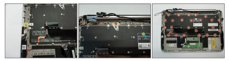
We removed the battery to avoid electric shocks. The hard disk, WiFi card, fan, touchpad and motherboard have also been removed.
