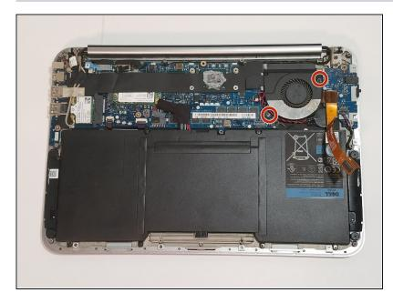
• Use a Phillips screwdriver to remove the two cooling fan screws.
