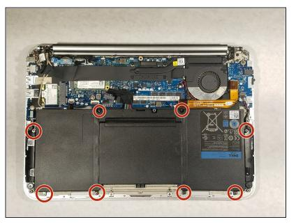
• Use a Phillips #00 screwdriver to remove the 8 screws that secure the battery.
