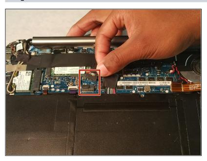
After the back panel has been removed, disconnect the battery to prevent electrical shock
