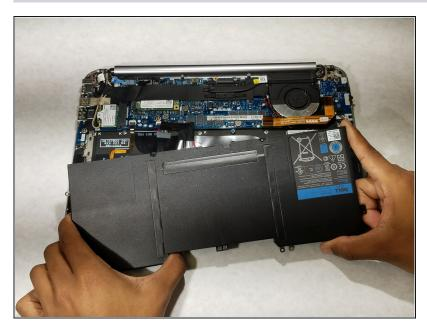
Once all the screws have been removed the battery is now safe to extract
