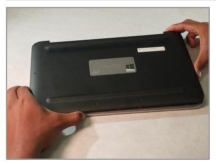
Carefully remove back panel after all screws have been removed.
