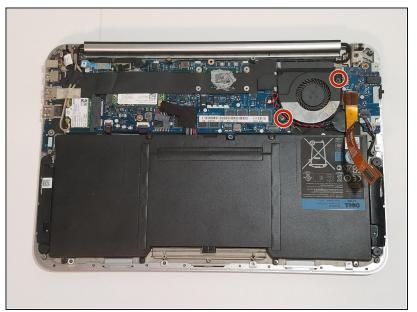
Use a Phillips screwdriver to remove the two cooling fan screws.
