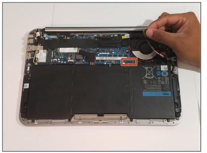
Disconnect yellow-colored ribbon cable from its port which sits at the bottom left of the fan housing.
