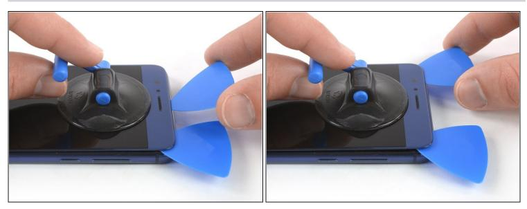
• Insert a second opening pick in the gap you created and slide it to the top left corner. Leave it in its place to prevent the adhesive from resealing.
