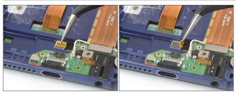
• Use a pair of tweezers to peel the grounding cable off of the midframe.
