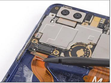
Use a spudger to pry up and disconnect the display flex cable from its motherboard socket.
