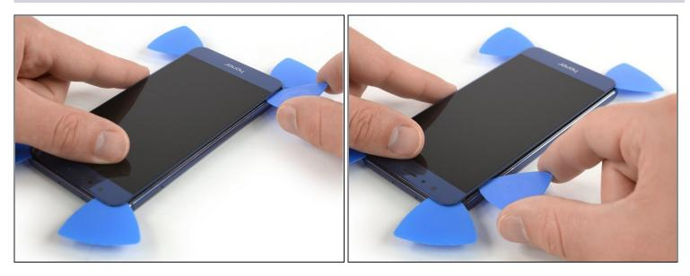
• Insert a fifth opening pick at the bottom left corner and slide it along the left edge of the phone to cut the remaining adhesive.
