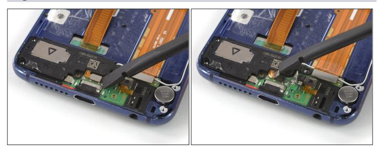
• Use a spudger to pry up and disconnect the loudspeaker flex cable.
