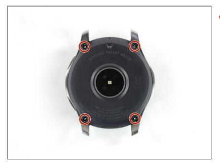
Remove the four Tri-point #00 screws (4.2 mm length) on the backside of the watch.
