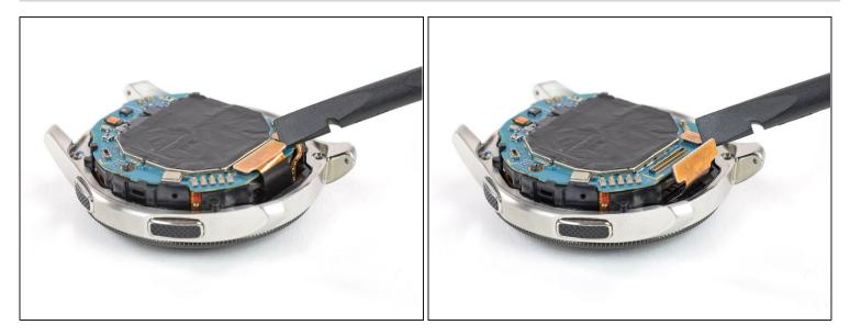
• Use a spudger to disconnect the display flex cable from the motherboard.
