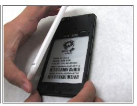
• Remove the back cover by inserting the plastic opening tool at the bottom left corner of the device.
