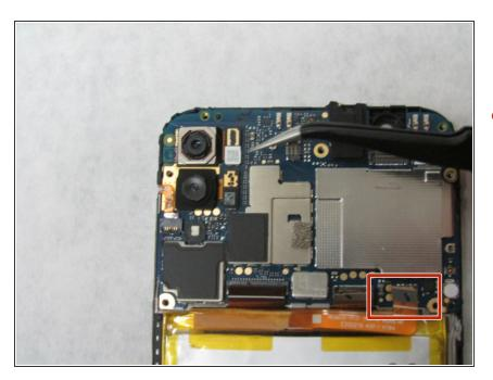
Disconnect the press fit connector located near the upper right corner of the battery to disengage the battery from the motherboard.
