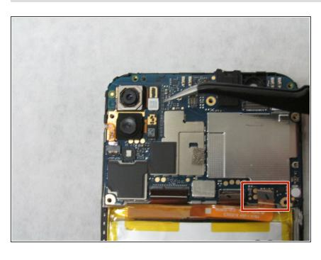
Disconnect the press fit connector located near the upper right corner of the battery to disengage the battery from the motherboard.
