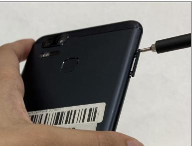
Use the sim card attachment for the screwdriver found in the IFIXIT box to remove the sim card tray from the phone.
