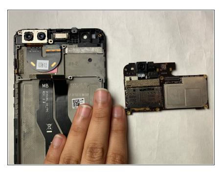
The finished product should be a motherboard with no connections to the body of the phone.
