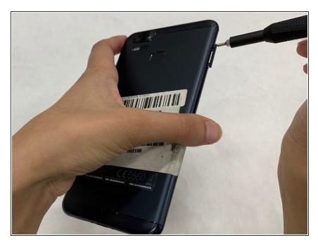
Use sim card attachment for the screwdriver found in the IFIXIT box to remove the sim card tray from the phone.
