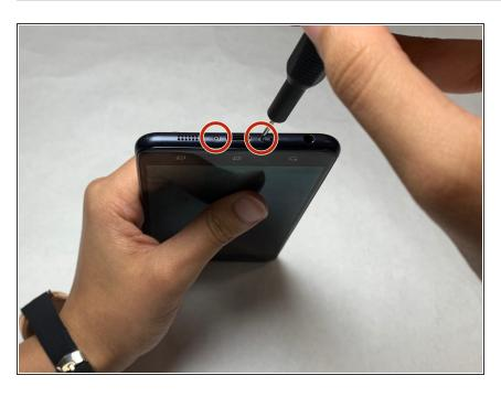
Remove the 3.5 mm screws on both sides of the charging port, on the bottom of the phone, using the T2 screwdriver.
