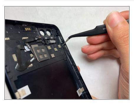
Use the angled tweezers to remove the power/volume buttons from the inside of the phone cover.
