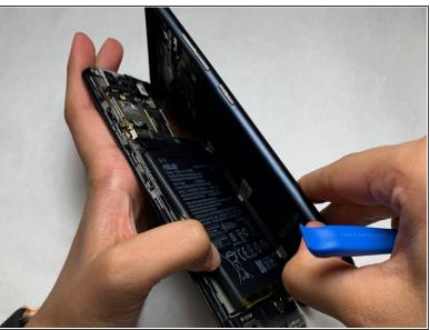
Use the opening tool to separate the screen and the plastic body of the phone.
