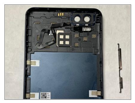
The finished product should be the volume and power buttons separated from the back casing of the phone.
