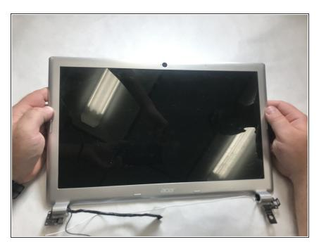
• Take the display assembly off and replace it with a new one.
