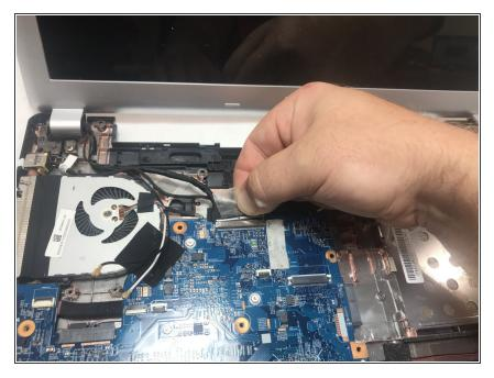
Gently disconnect the display cable connector between the display assembly and the motherboard.
