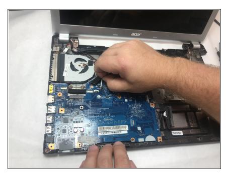
• Remove the tape holding down the display cable that connects it to the motherboard.
