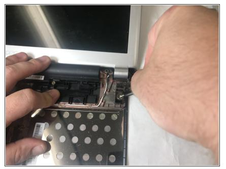
• Using a #0 Phillips screw driver, remove the other 2.5 mm by 5 mm phillips screw that holds the display assembly.
