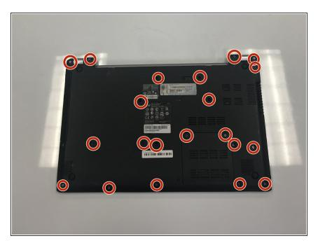
• Use a #0 Phillips head screw driver to remove all of the screws.
