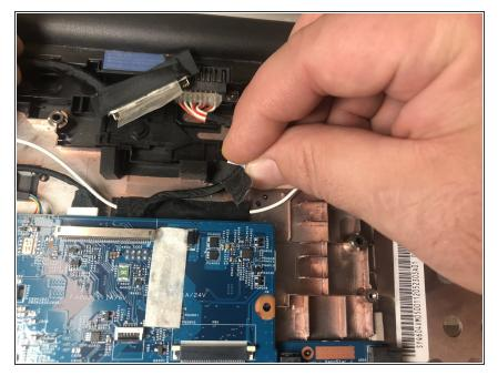
• Disconnect the tape that is holding the white antenna cable to the motherboard.
