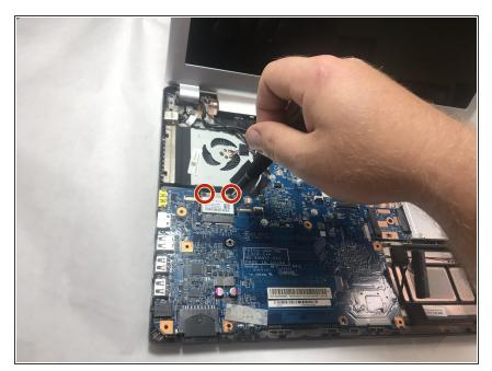
Use #0 Phillips screw driver to remove the two 2.5 x 5 mm Phillips #0 screws connecting the Wi-Fi card to the Motherboard.
