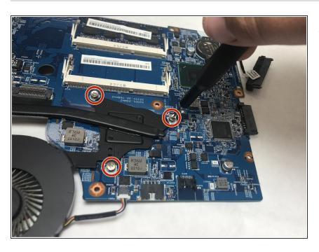
Use #0 Philips screw driver to unscrew the three 2.5 mm x 4 mm screws connecting the CPU fan to the Motherboard.
