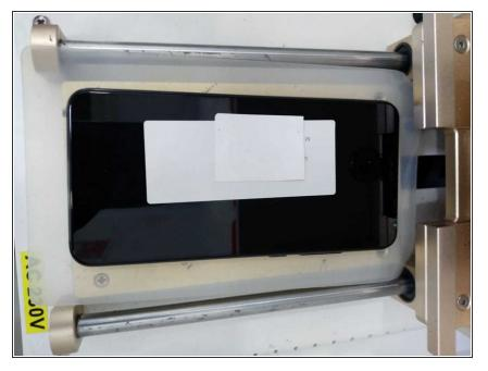
Place on top of a hot plate on soften the adhesive on the back cover (no more than 90°c of heat). You can also use a heat gun, but be careful not to overdo it.
