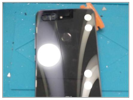
Use a razor or a piece of plastic to take off the cover. Watch out! It is very fragile, use a lot of caution. Be careful with the flex cable. Do not insert the blade too far or you can cut it.
