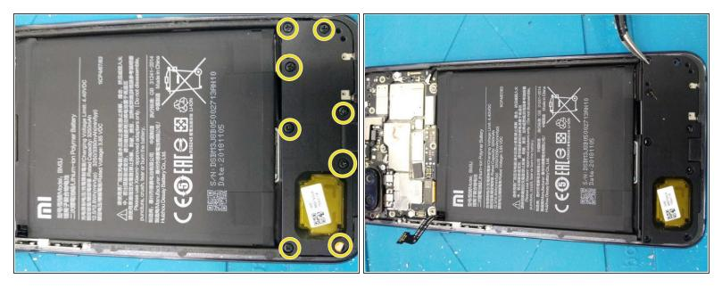
Unscrew the eight screws that fasten the bottom speaker. This step isn't necessary but it makes it much easier to pull the adhesive on the battery.
