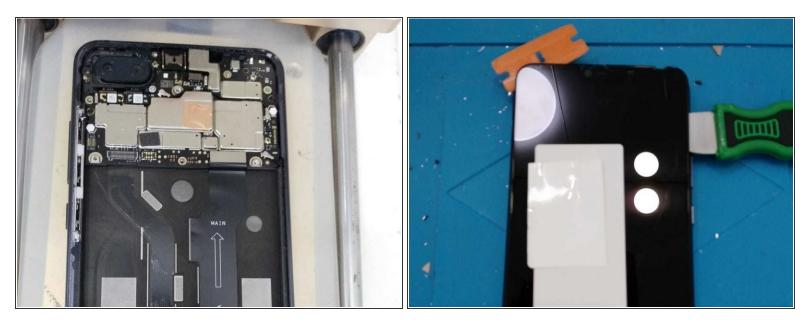
Place the screen on the plate (apply heat), separate the screen from under as you have done with the back cover
