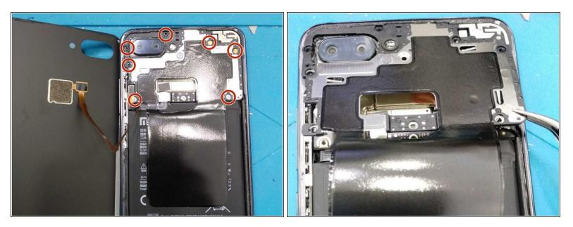
• Lift the cover from right to left, but do not do it completely while the flex cable is still connected. Unscrew the seven screws and place them as in the image.
