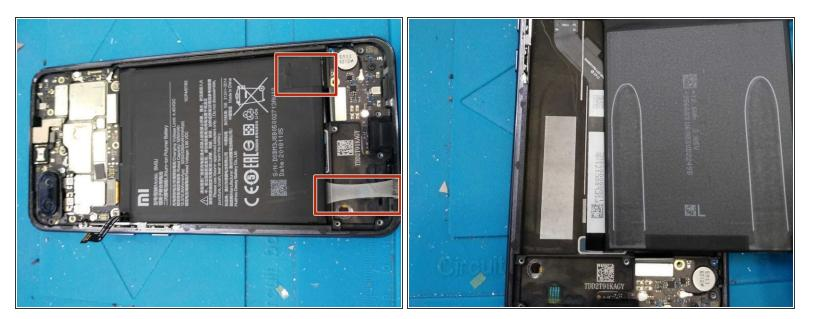
• Carefully pull the two adhesives that attatch the battery to the middle frame.
