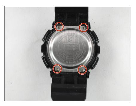
Remove the four Phillips #00 screws from the back of the watch.
