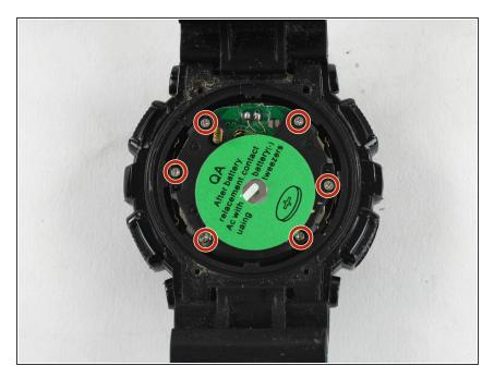
Remove the six Phillips #00 screws from the inside of the watch.
