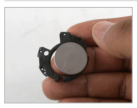
Use your finger to push the CR2025 Lithium battery out of its protective casing.
