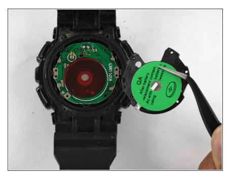
Use a pair of tweezers to remove the protective casing with the battery attached to it.
