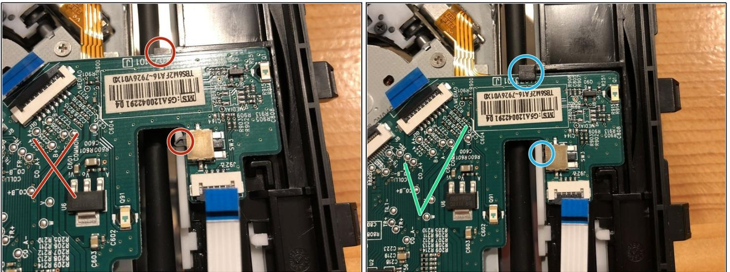
⚠ When installing the new PCB, look out for the spots as shown in Photo 1 (red circles). When you follow photo 1 and tight it with screws, you could break the PCB ! So do the opposite of Photo 1!
