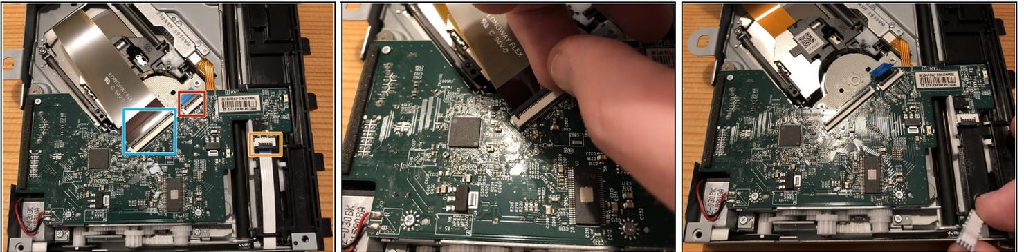
**⚠ Do NOT remove the ribbon cables yet, make sure you opened up the ZIF connector first and then remove the ribbon cables. Otherwise you could damage the PCB.**
