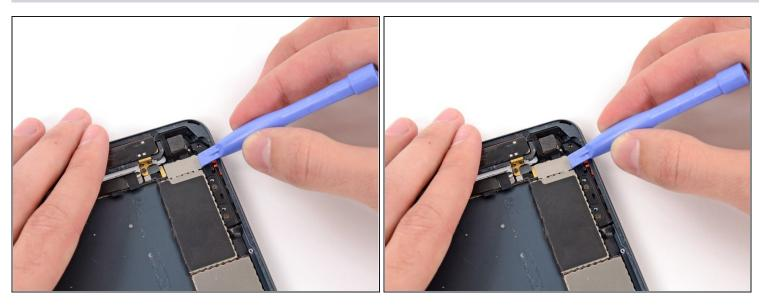
Use a plastic opening tool to push the bracket slightly to the left.
