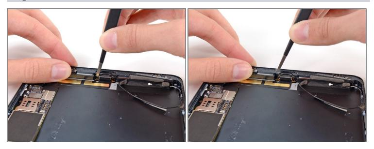
• Use <u>tweezers</u> to remove the small plastic cover on top of the horizontal screw on the right side of the Lightning connector housing.
