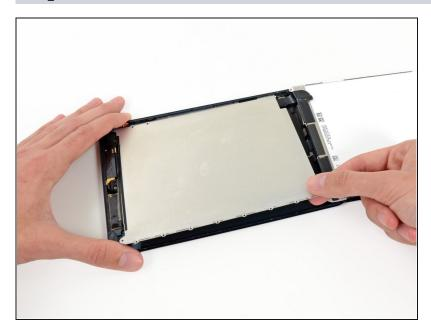
• Remove the LCD shield plate from the iPad.
