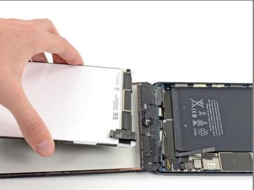
Lift and remove the LCD from the iPad Mini.
