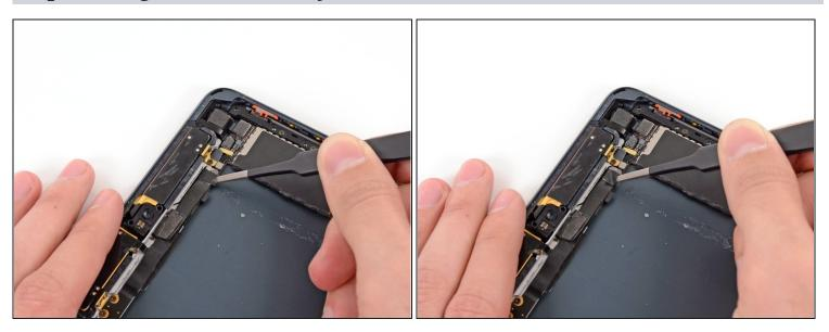
• Use <u>tweezers</u> to peel up and remove the small piece of tape covering the front-facing camera cable connector.
