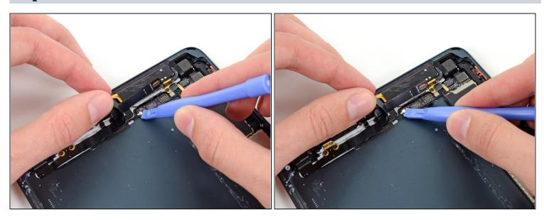
• Use a plastic opening tool to pry the top left antenna cable up from its socket on the logic board.
