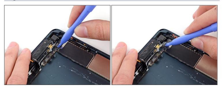
• Pry the top right antenna's ribbon cable up from its socket on the logic board with a plastic opening tool.
