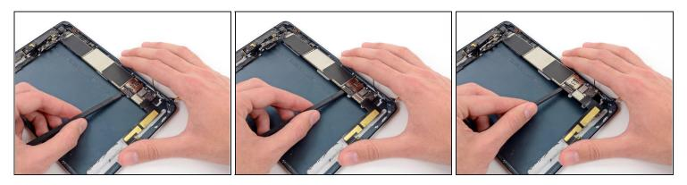
• Continue to use the spudger to pry the logic board up from the rear case.
