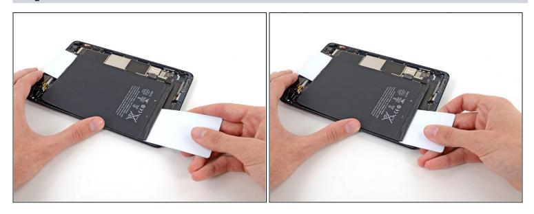
• Insert a second plastic card beneath the bottom left corner of the battery.
