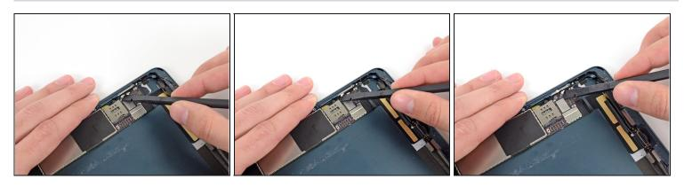
• Use the flat end of a spudger to disconnect the two bottom antenna cable connectors from their sockets on the logic board.
