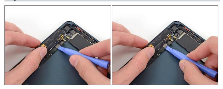
• Use a plastic opening tool to pry the headphone jack cable's connector up out of its socket on the logic board.
