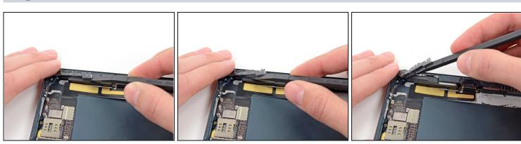
• Use the flat end of a spudger to loosen the foam adhesive holding the antenna to the right speaker.
